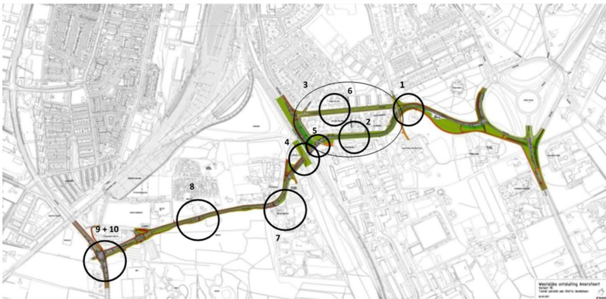
Figure 8. Map of scenario 7B (2015) with indicated changes. For the areas with a circle indicate the area that changes, compared to scenario 7B (2013), will occur. Source: *Verbetering doorstroming verkeer aan de westzijde van Amersfoort, uitwerking coalitieakkoord. Gemeente Amersfoort (2013).*
